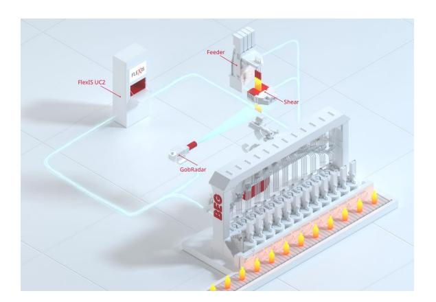
Gob Control Closed Loop Integral part of SMARTFEEDER™
