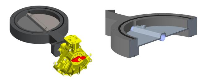
The 3.1 bar air consumption of the butterfly valve is 0.226 liters/cycle against 0,8 liters/cycle for the previous actuator. This approximately corresponds to 72% in savings on compressed air.
