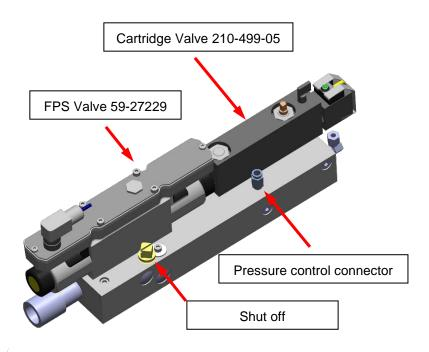
from the top of the valve block. The air supply to the block is direct from the manifold. The exhaust is partially going into the exhaust manifold and partially into the atmosphere. The needle on the exhaust valve controls the exhaust air coming back from the plunger up line. The cartridge valve is identical to the NC valves used in the 26 line Valve Block, on the Universal Conveyor Valve Block and on the NIS PCM blank side.
