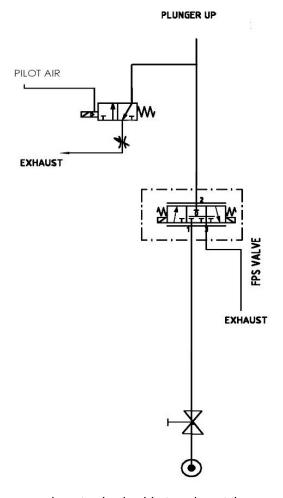
(NO) valve to force the plunger down in MS. This means the plunger up exhaust valve is able to exhaust the leakage air which is flowing into the plunger up cylinder from the plunger down pressure and avoids the creeping up of the plunger while all valves de-powered.
