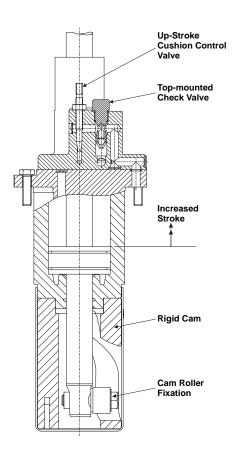
Two-way air operated Funnel Mechanism 200-2100
